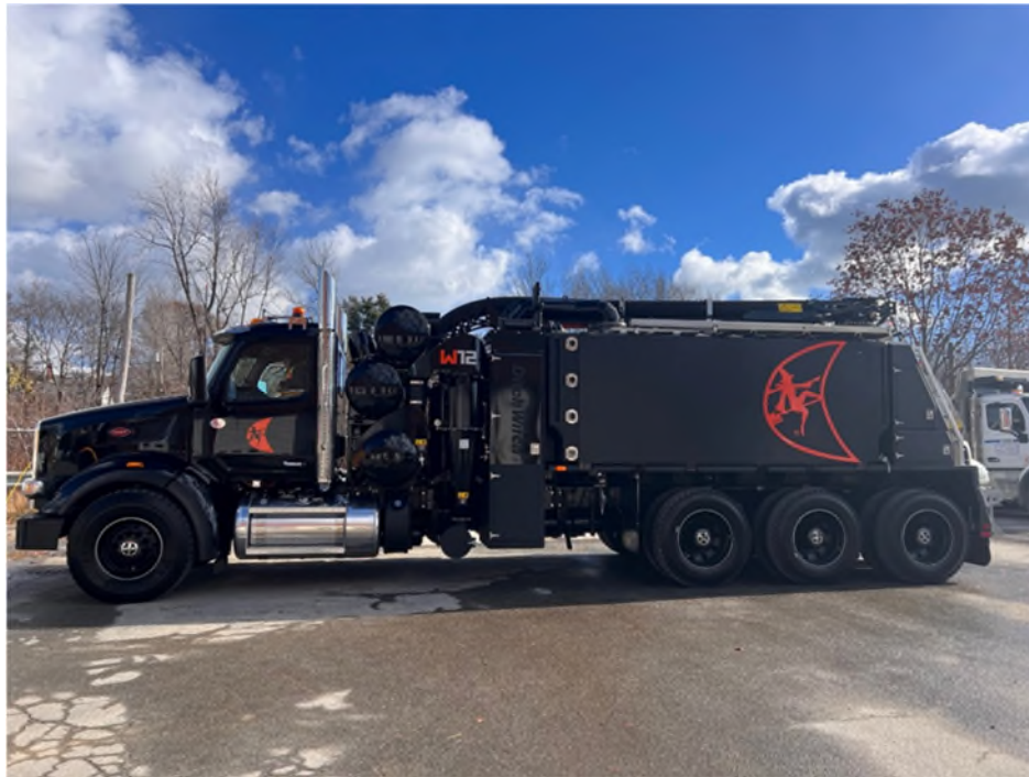
Portland Water District Ditch Witch W12 Vacator
